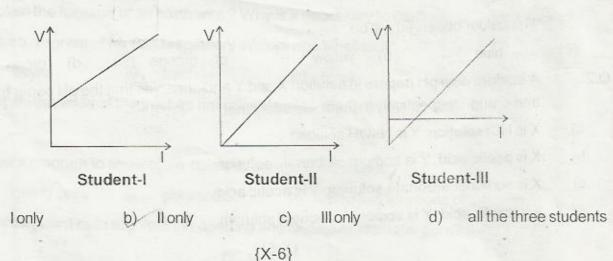
Q.33 The current flowing through a resistor connected in an electric circuit and the potential difference developed across the ends of it are as show in the diagrams.
